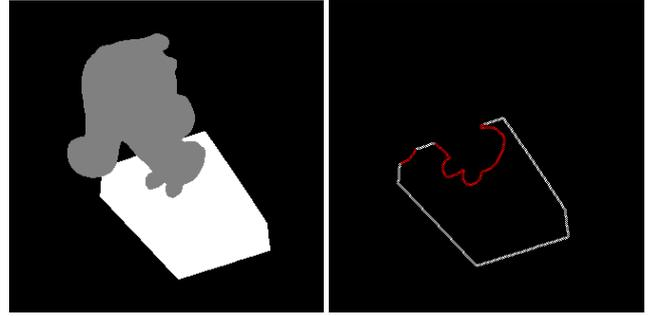
**Figure 5:** Occlusion handling when tracking multiple objects. Left: Common silhouette mask  $I_s$ , which is generated by rendering each object model with a unique color equals to its object index. A box is occluded by a squirrel in the scene. Right: The projected contour points of the box object. The occluded contour points (marked as red) are discarded in pose optimization.
