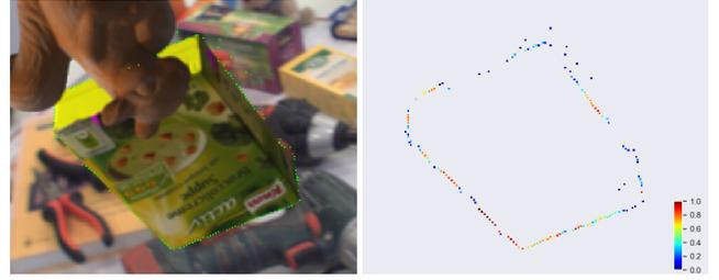
**Figure 4:** Left: Searched object contour points  $\mathbf{s}_i$  (green dots) in the video frame. Right: The confidence  $w(\mathbf{s}_i)$  of object contour point  $\mathbf{s}_i$ .
